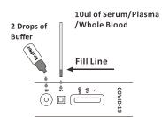
To use a dropper: Hold the dropper vertically, draw the specimen up to the Fill Line (approximately 10µI), and transfer the specimen to the specimen well (S) of the test cassette, then add 2 drops of buffer (approximately 80µI) to the buffer well (B) and start the timer. Avoid trapping air bubbles in the specimen well.
